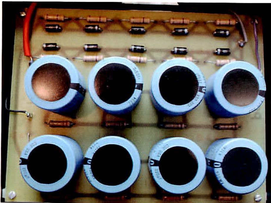
This is a typical voltage doubler power supply rated up to 3200 volts
