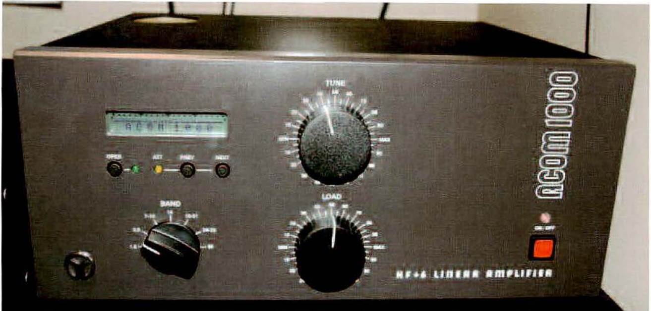
Front Panel layout of the Acom 1000
