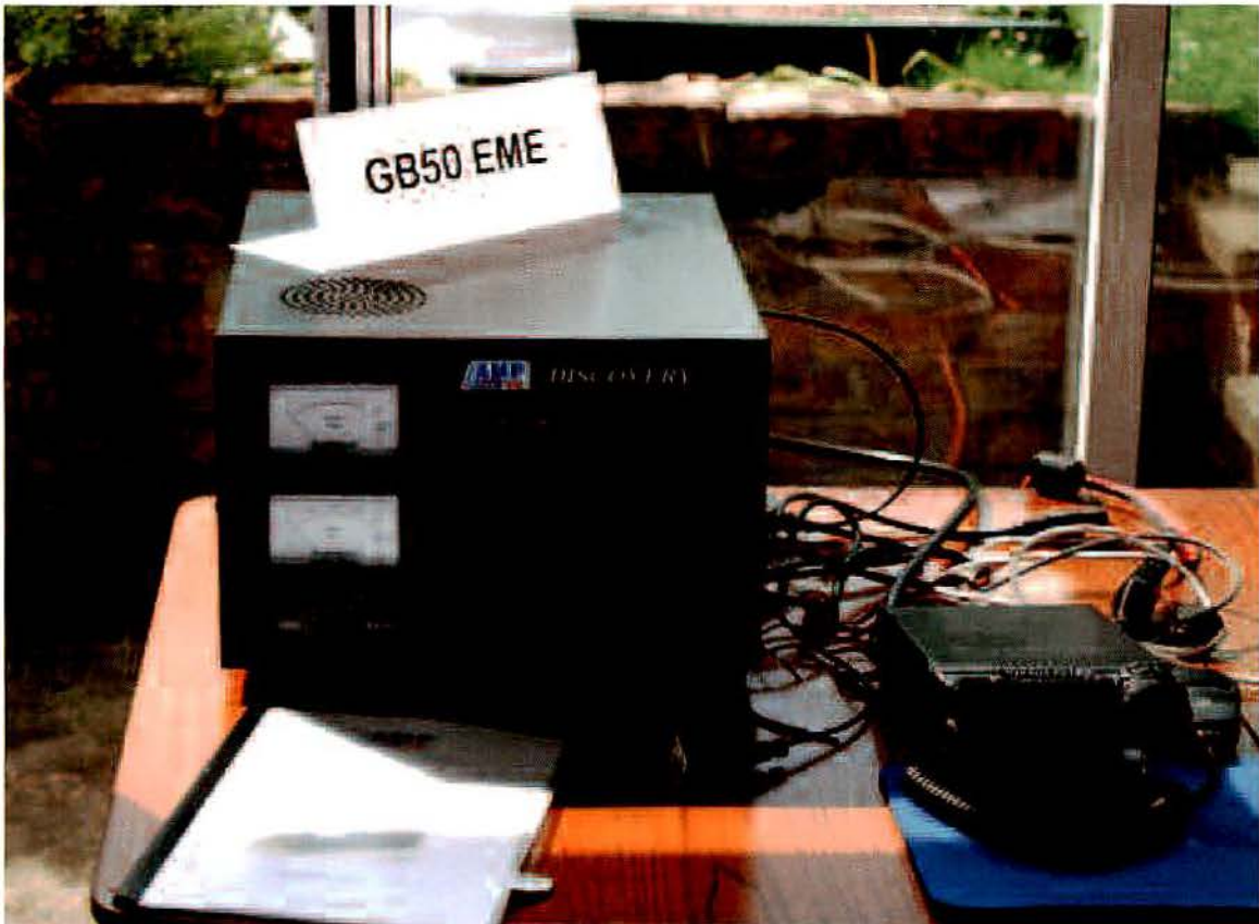
Transmission Frequency 432.065 Using only a IC706 and a 70cm Discovery to work 480,000 miles
