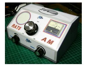
Excellent example built by Eric GW8LJJ for club demonstration. *(in this build the controls are not directly soldered to the PCB)*
