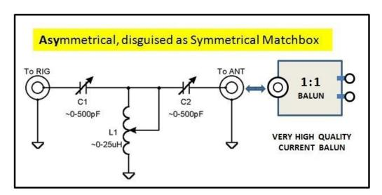
**It's not bad, but it's not great.** However with this circuit I was able to run one kilowatt without burning my fingers on the key, or my lips on the mic. A prerequisite for this is, you have to have a good matchbox which has no problem dealing with the high voltage due to the higher impedance when not using the 4:1 transformation in front of it. The variable capacitors should be rated about 6KV or more.
