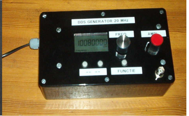
DDS Generator build in a box.
