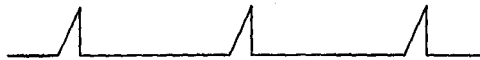
FIG. 15-51.—Wave form of sweep voltage used when it is desired to observe only a portion of the cycle of voltage impressed upon the oscilloscope.
