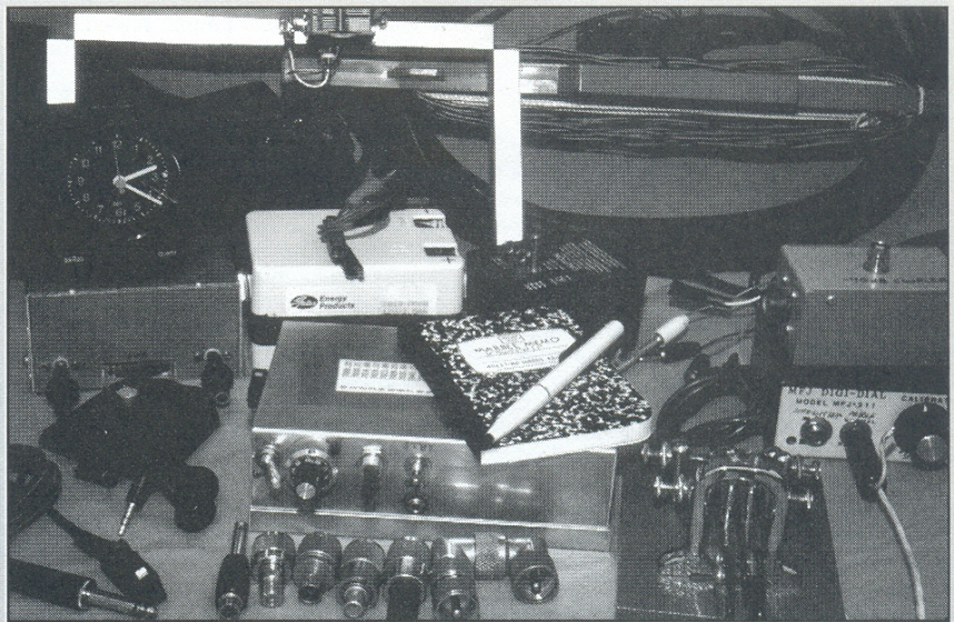
Fig F—KB6FPW: This is the entire 40-40 accessory lineup. This stuff isn't used all at once, but I draw upon these items to satisfy various operating requirements such as business or camping trips, trips to visit relatives, RFI investigation, or operation at home. I've even operated mobile. Progressing from lower left to upper right are pictured remote microswitch hand key; ear buds in carrying case; spare final; SWR bridge/Transmatch with removable knobs; Braun QRP station clock; adaptors 1/4 inch to RCA, UHF to F, BNC, RCA and five-way banana; UHF U-turn consisting of two elbows and one male-male adaptor; the 40-40; log book; pen; Gates Cyclon 12 V/2.5 Ah six-pack; banana to alligator clip pair; shaving kit bag (black); tuned, shielded loop; Vibroplex iambic paddle; homebrew Curtis keyer in a gutted MFJ aluminum box; -20 dB coupler; RCA patch cord; Ault Model 5000 12 V/300 mA wall cube; lastly, in the back, a 40-m dipole with 50 feet of coaxial feed line and choke-style balun wound on an extension cord holder.
