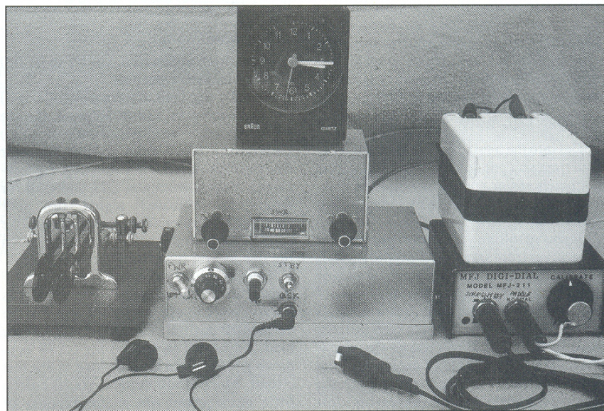
KB6FPW: Reversing the view, we see the user controls for the rig and Transmatch. Earbuds are connected and ready to go, as well as the remote microswitch hand key.
