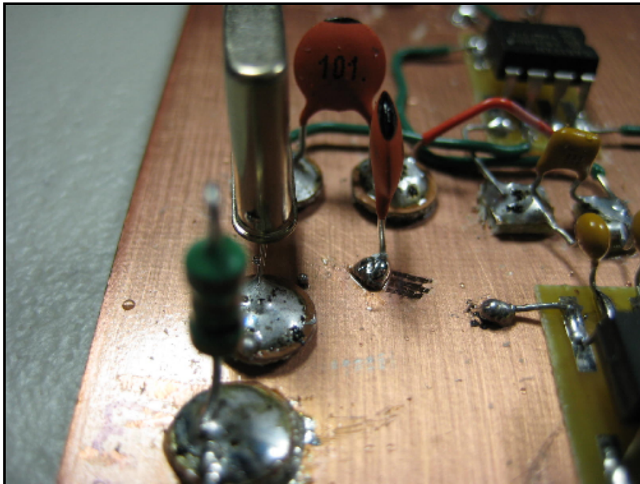
The crystal frequency is needed on pins 6 & 7 of the SA602 mixer.
