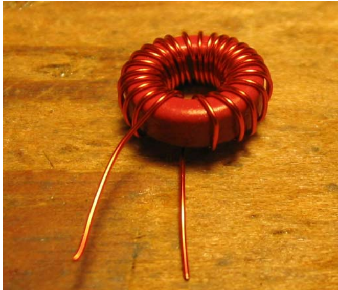
This picture shows a T37-2 with 24 Turns of # 28 wire.
