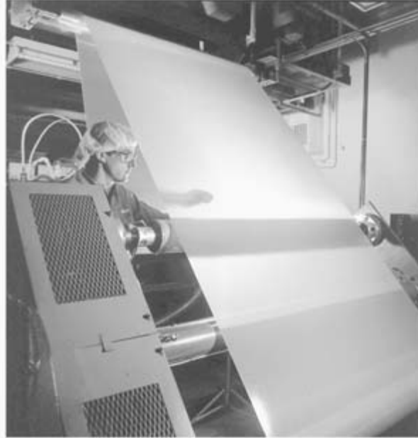
FIGURE 7.3 Prepreg after treatment with resin. (Photo courtesy of ParkNelco.)
