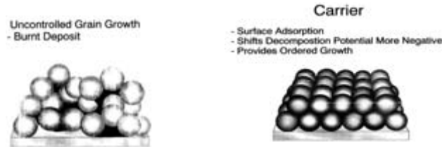
FIGURE 29.7 The effect of a carrier on the grain structure of the deposited copper.
