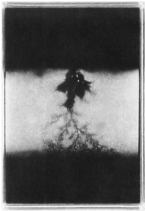
FIGURE 53.10 Transmitted light micrograph through a PCB that failed in the field. Dendritic growth has formed at the interface of a UV-cured screened solder mask and the FR-4 surface.
