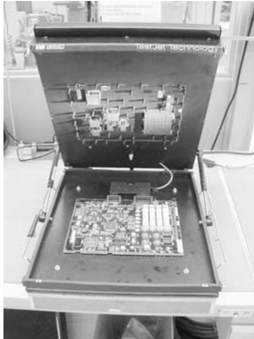
FIGURE 52.14 A test fixture with board on a bed of nails, with clamshell top fixture containing capacitive sensor plates. Notice eight closely spaced sensor plates (right) that test for opens in eight (white) connectors on the board.
