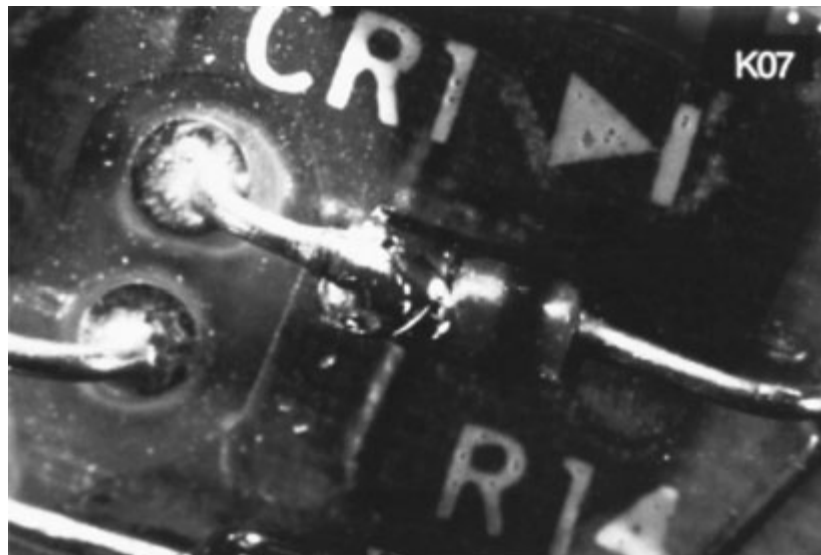
FIGURE 49.19 Damaged axial leaded component. (IPC.)
