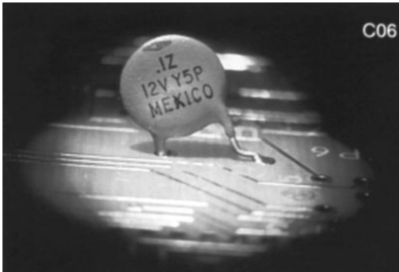
FIGURE 49.21 Radial component coating meniscus in the PTH. (IPC.)
