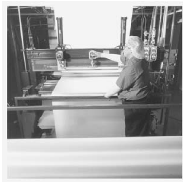
FIGURE 7.2 Fiberglass cloth being fed into a treater. (Photo courtesy of ParkNelco.)
