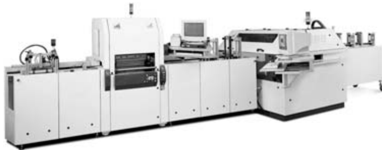
FIGURE 38.13 Integrated sequential test system. (Courtesy of atg Test Systems GmbH).
