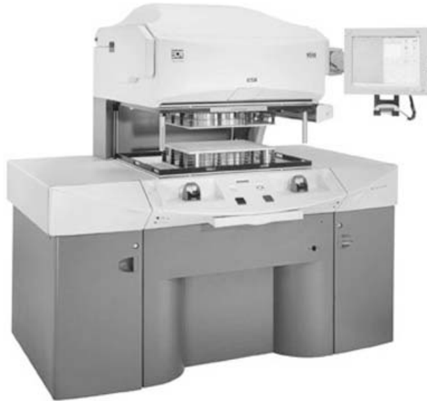
FIGURE 39.3 Universal grid test system. (Courtesy of Everett Charles Technologies.)
