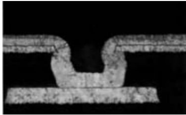
FIGURE 29.2 Horizontal PTH/Pulse-Plated Resin-Coated Copper™ microvia.
