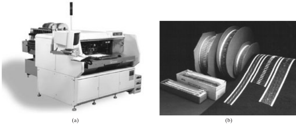
FIGURE 41.2 Axial led components in various assembly formats. (a) Automatic axial inserter. (b) Axial led components.
