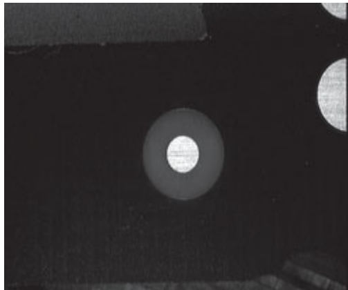
FIGURE 41.10 A typical fiducial on a printed wiring board.
