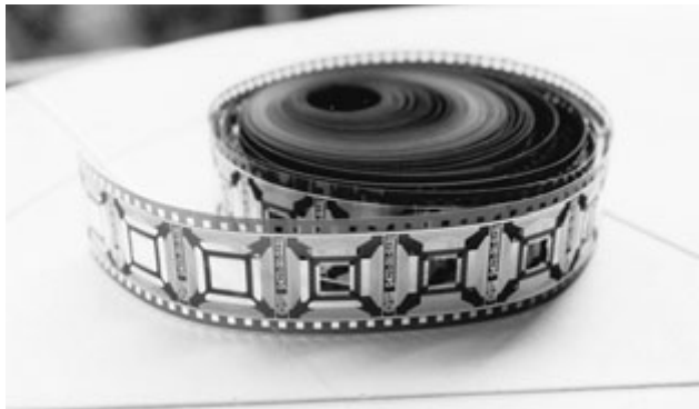
FIGURE 56.2 TAB circuits. (Courtesy of Shindo Denshi.)
