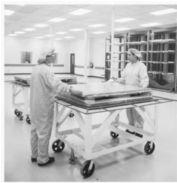
FIGURE 7.4 Prepreg layup. (Photo courtesy of ParkNelco.)
