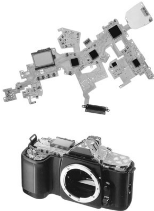
FIGURE 56.3 Main flexible circuit of a camera. (Courtesy of Nikon.)
