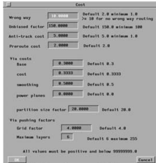
FIGURE 21.6 Example of autorouter menu for an advanced CAD system. Tuning an autorouter can adjust the way it will design HDI boards.
