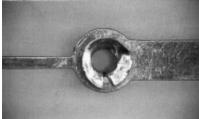
FIGURE 49.10 Rivet swage split into barrel. (IPC)
