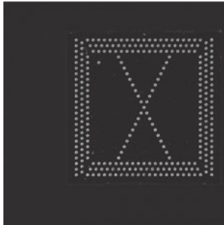
FIGURE 41.12 An image of flip-chip bumps as viewed by a vision system.
