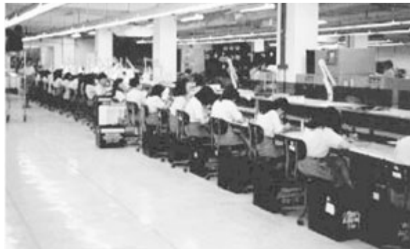
FIGURE 41.21 Manual printed circuit assembly line.
