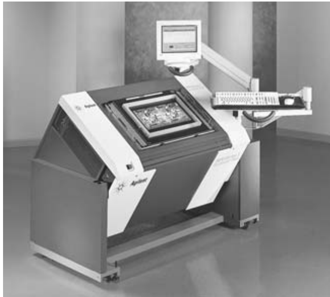
FIGURE 52.10 Example of a commercial in-circuit test head and operator terminal, with a printed circuit board mounted in the testing position on top of the bed-of-nails fixture.
