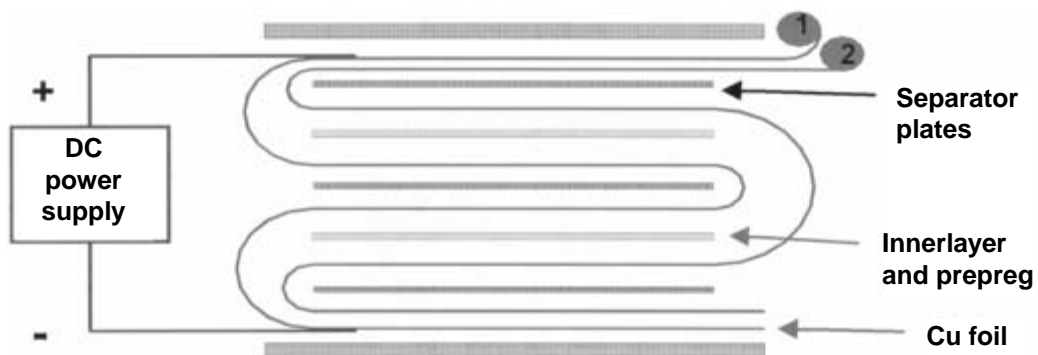
FIGURE 7.8 Laminate pressing with continuous copper foil and direct-current heating. (Illustration courtesy of Cedat.)
