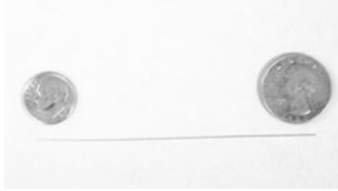
FIGURE 40.1 Tapered pin for fine-geometry fixture.
