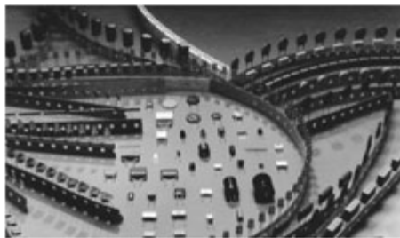
FIGURE 41.3 Radial led components in various assembly formats.
