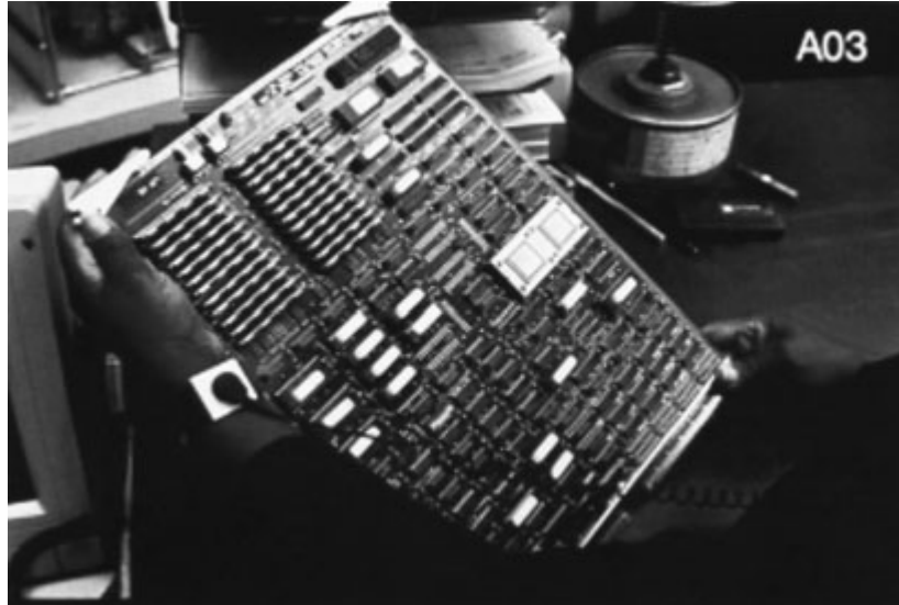
FIGURE 49.2 PCBA edge handling. ( IPC. )
