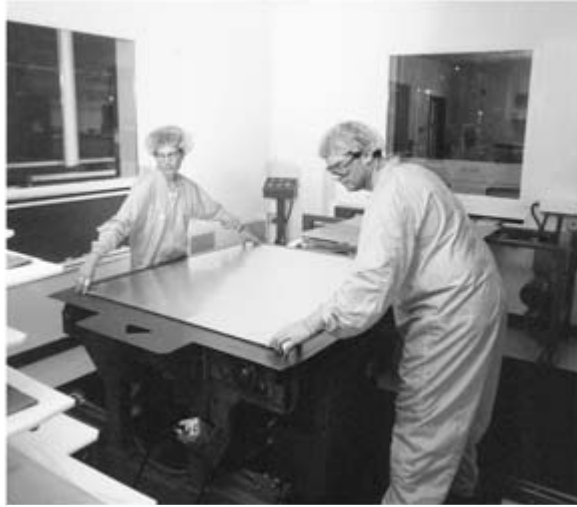
FIGURE 7.5 Laminate setup for pressing. (Photo courtesy of ParkNelco.)
