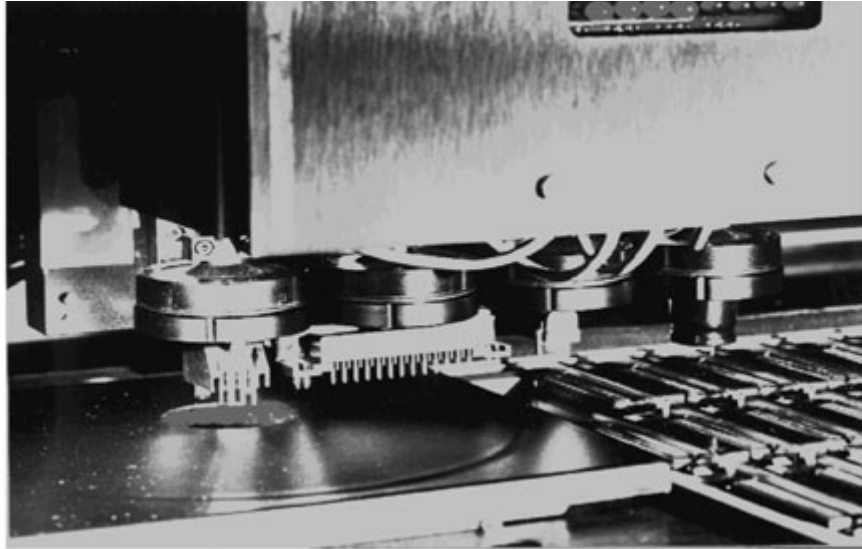
FIGURE 41.29 Odd components being inspected over vision system.
