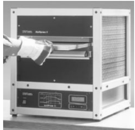
Fig. 11.5 Typical lamination press for multi-layer boards (Muller, 2000)
