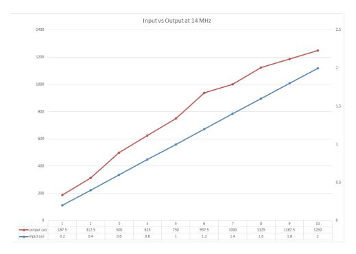
Don't hold me to the very low drive power readings at .2 and .4w, I was using my Elecraft KX3's power settings to measure that, and the accuracy is good, but not perfect. Still, it looks like 1db compression happens at about 85% of full output. In this case, and on this band, that's at about 1062w out (85% of 1250w). By now you've probably noticed that you can drive this to full output with an average of just 2 or 3 watts.
