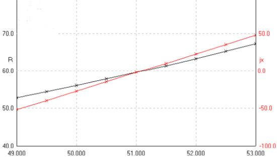
Figure 8 Input impedance of 'wide' antenna
