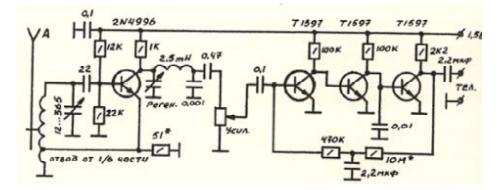
Data for L the same as for above receiver. Tap made from 1/6 parts of the L. Resistor on \*51 Ohm should be pickup for used band (or, the same, used L). Inductor for 2.5 mH is home brew, it contains 200 turns onto a ferrite ring 20x12x4 mm, permeability 600. Transistor used in regenerative stage should be good RF transistor with f = 300 MHz, and gain =100 and more. Any audio transistors can be used in audio amplifier.
