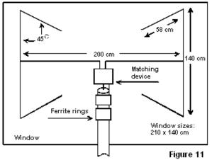
Figure 11 A window dipole antenna with capacitive loads of central installation
