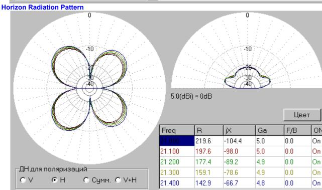
Comments: Antenna has strong vertical radiation. A good pattern in the vertical plane. Antenna has almost egg shape pattern dropped to four lobes in horizontal plane, so, it demands to choose a proper direction before an installation of the antenna. Antenna provides DX QSOs. Antenna has Z= 177- j89-Ohms at 21200kHz. Any ATU does good matching for such load.
