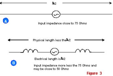
Figure 3 A shortening and full size dipole antenna
