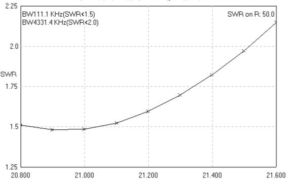
antenna with electrical length in  $\lambda/2$  (having physical length bit less then  $\lambda/2$ ) has input impedance less them 75 Ohms and maybe, close to 60- 50-Ohms, see **Figure 3B**. So, for feeding a dipole trap antenna a 50-Ohms coaxial cable can be used with a high efficiency.
