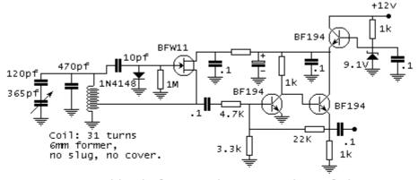
VFO: Use two identical VFOs using two sections of the broadcast gang, switch power suppy for each VFO. The 470Pf should be a polystrene or a 'Styroflex' cap. The 14 Mhz VFO tunes from 4 to 4.4Mzh.
