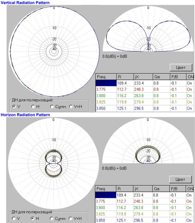
**Comments:** Antenna radiates mainly radio waves with vertical polarization. A very good pattern with low lobes in the vertical plane. Circular pattern in horizontal plane. It is fine for DX- QSO. Antenna has Z= 116+ j263-Ohms at 3800-kHz. Almost any ATU does good matching for such load.
