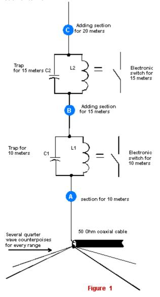
Figure 1 A ham vertical trap antenna
