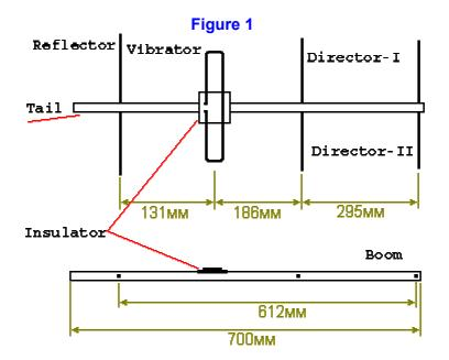
The design of antenna vibrator is shown on Figure 2. Coaxial cable has 850-mm length and this one goes along the boom. Soldered place must be protected from weather.
