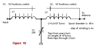
But scheme in **Fig. 10** has advantages. At first, it is much easier to use only one grounded high-quality capacitor instead of two ones but insulated from metal cabinet. Secondly, it is wise to substitute expensive inductor with slide control to two cheapie spools with taps.
