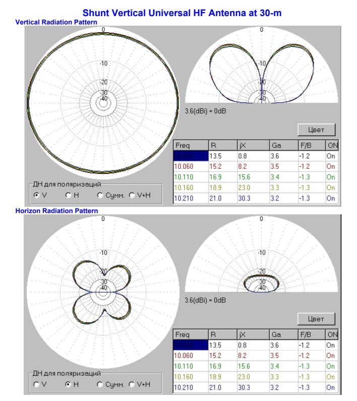
**Comments:** Antenna has strong vertical radiation. A good pattern in the vertical plane. Antenna has strong radiation at high corners that allows to do local QSOs. Antenna has almost circular pattern in horizontal plane. Antenna provides DX and local QSOs. Antenna has Z= 16.9+ j15.6-Ohms at 10110-kHz. Any ATU does good matching for such load.
