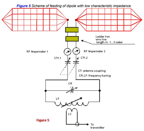
circuit 'LF- CR', that is coupled with help of coupling coil 'LC' with a transmitter. With the help of variable
