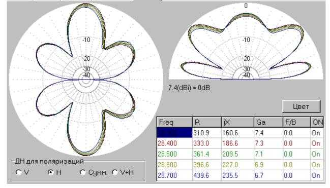
**Comments:** Antenna has strong horizon radiation. For the horizon radiation antenna has a not bad pattern in the vertical plane, and "eight- figure" pattern dropped to lobes in the horizon plane. Antenna can provide DX QSOs at the horizon radiation. Antenna has impedance 396+j227-Ohms at 28600-kHz. Not all ATUs do good matching for such load.
