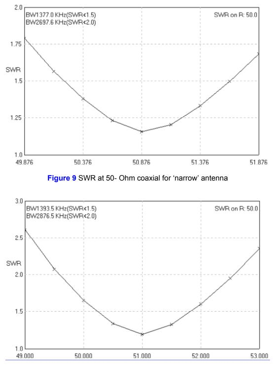
Figure 10 SWR at 50- Ohm coaxial for 'wide' antenna
