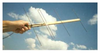
Figure 1 shows a design of such antenna. The boom is made of a wooden strip.. Elements and the vibrator are made of 2-mm copper wire (# 12 AWG).
