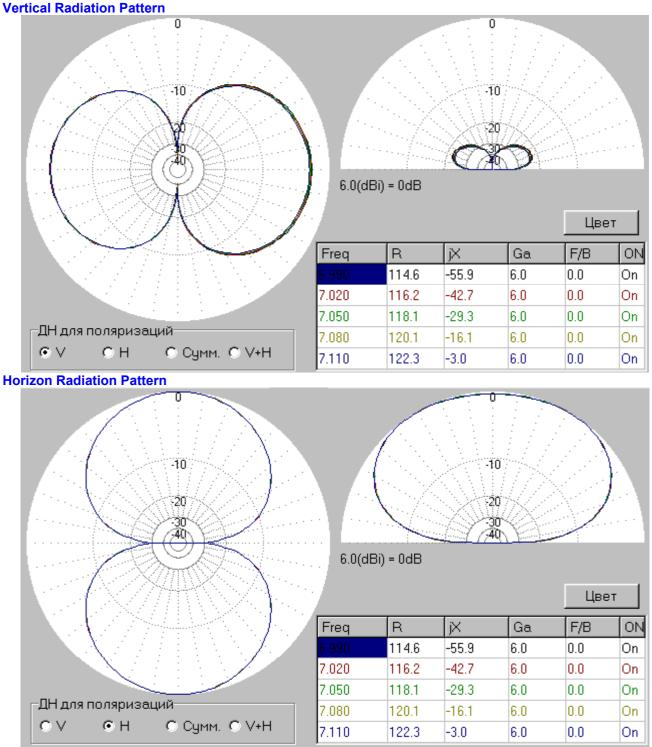
**Comments:** Antenna radiates mainly radio waves with horizontal polarization. A good pattern in the vertical plane. Antenna has strong zenith radiation that allows to do local QSOs. "Eight- figure" pattern in horizontal plane, so, it demands to choose a proper direction before an installation of the antenna. Antenna is fine for DX and local QSOs. Antenna has Z= 116+ j263-Ohms at 3800-kHz. Almost any ATU does good matching for such load.
