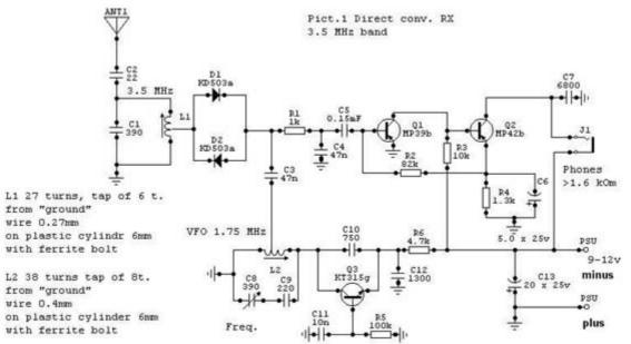
Alongside to this 80m variant receivers under the similar circuit on 40 and 20 m bands are also were constructed. The results were obtained also excellent.
