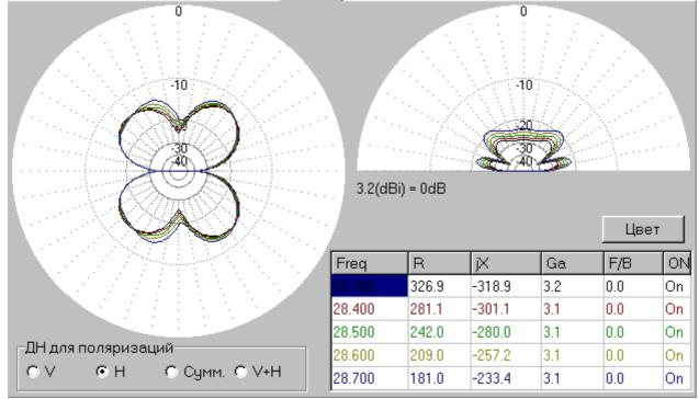
**Comments:** Antenna has strong vertical radiation. A not bad pattern in the vertical plane. Antenna has a four- shaped lobes pattern in horizontal plane, so, it demands to choose a proper direction before an installation of the antenna.. Antenna can provide DX QSOs. Antenna has Z= 242- j280-Ohms at 28500-kHz. Any ATU does good matching for such load.
