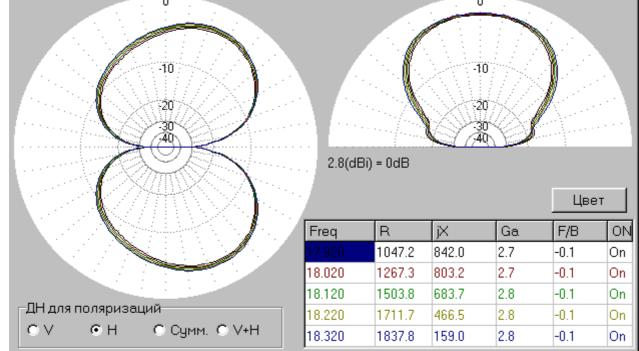
**Comments:** Antenna has both, a strong vertical and strong horizon radiation. For the vertical radiation antenna has a good pattern in the vertical plane, and almost circular pattern in the horizon plane. Pattern for horizon radiation is not so good as to vertical polarization. Antenna can provide DX QSOs at vertical and horizon radiation. Antenna has impedance 1711+j466-Ohms at 18220-kHz. Not all ATUs do good matching for such load.
