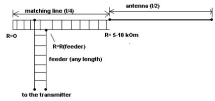
The feeder from the transmitter with a specific impedance  $R_f$  is connected to the matching line in the point, where impedance of the latter is equal to that of the feeder. Such point is usually located not so far from the shortened end. If everything is done properly, feeder may have any length and SWR is closed to 1:1 in rather narrow band, central frequency of which is determined by the geometrical size of matching line and antenna.
