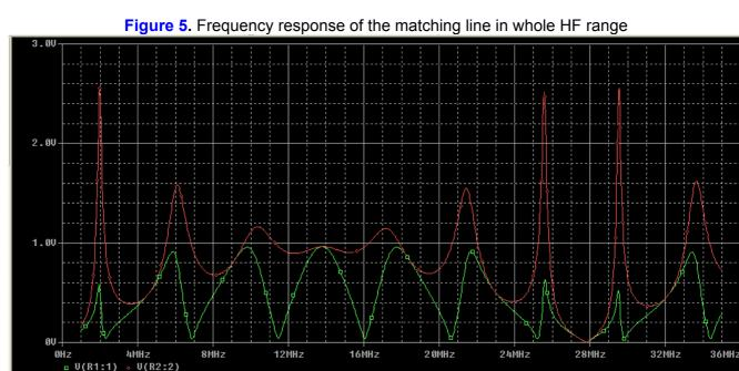
I guess, that these results may be assumed at least as a qualitative explanation of the antenna behavior. I say "qualitative" because the whole system can not be adequately represented by a matching line with a resistor at the end – impedance of the antenna wire also should be taken into account. However it is clear, why besides 'native' band, antenna works well on 21 MHz, and why on frequencies about 28500 there is a minimum of performance, which rapidly increases when moving up to 29 MHz.
