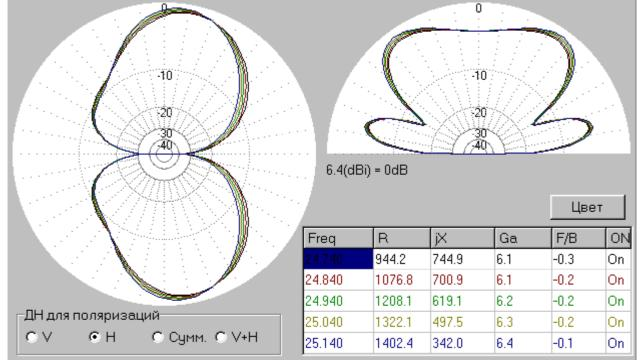
**Comments:** Antenna has strong horizon radiation. For the horizon radiation antenna has a not bad pattern in the vertical plane, and "eight- figure" pattern in the horizon plane. Antenna can provide DX QSOs at horizon radiation. Antenna has impedance 1208+j619-Ohms at 21200-kHz. Not all ATUs do good matching for such load.
