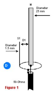
Open Sleeve antennas presented at this article were designed by UA3AVR (Reference: Dmitry Fedorov (UA3AVR).: Multi-range vertical Open Sleeve.- Radiomir. HF and VHF, 2001, #8, pp. 34-36). Table 1 shows data for the Open Sleeve Figure 1 shows the design of the antennas
