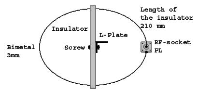
Antenna has weight of 900 gram. SWR is: at 430-MHz =1.2:1, at 435-MHz =1:1, at 440-MHz=1.3:1 SWR was metered by device SWR-121. If you will use boom
