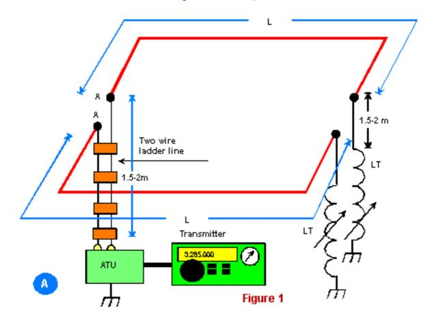
Figure 1 Tuned dipole
