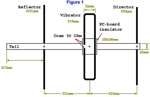
A 50-Ohms coaxial cable is used with the antenna without any symmetrical devices. The cable goes along the boom and get out from the tail. For antenna folding you can loose screws, turn antenna vibrator along the boom, and again strength the screws. Antenna director and reflector is removed from the boom and hide inside the boom.
