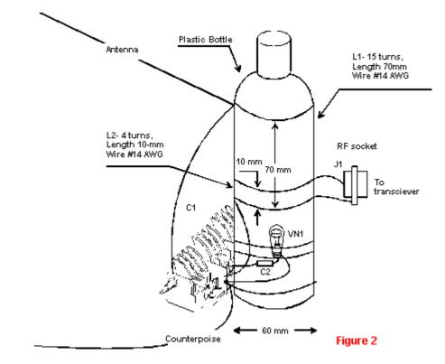
L2 is placed at the bottom of L1. L2 contains 4 turns of copper wire in diameter of 1,5 millimeters (# 14 AWG), length of winding is 10 millimeters. Ends of L2 are directly soldered to J1 RF – socket. VN1 is attached by a piece of Scotch to the bottle. Antenna is tuned by max glow of VN1.
