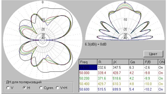
**Comments:** Antenna has horizon and vertical radiation. For the horizon radiation antenna has a not bad pattern in the vertical plane, and "eight- figure" pattern dropped to lobes in the horizon plane. Antenna can provide DX QSOs at horizon radiation. Antenna has impedance 429+j599-Ohms at 50600-kHz. Not all ATUs do good matching for such load.
