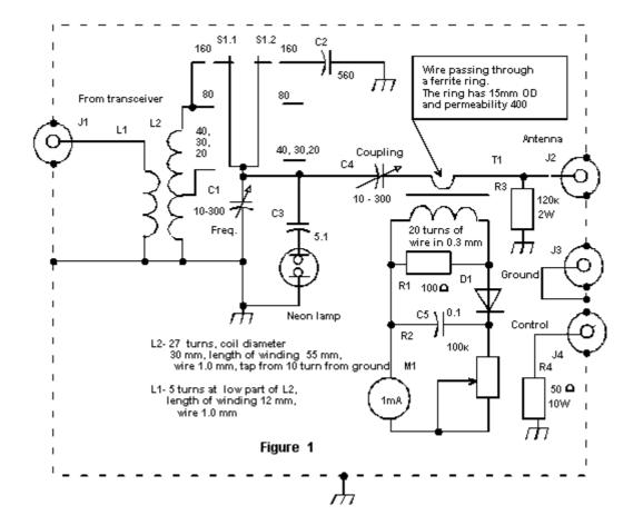
Certainly, when tank L2C1 (see **Fig.1**) is tuned in resonance with the input frequency, a high RF voltage is on the tank, and a little part of the RF energy from the tank L2C1 is induced on the dummy load R4. Hence, a small RF voltage is presence on R4, and a very little power goes in the antenna. Off course, a little RF energy also is induced on current transformer
