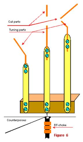
Vibrators have length  $(\lambda/4)^*(0.5-0.9)$ . Each vibrator is matched with coaxial cable with help of its own a 'lengthening' coil. You can use this design if you have a lack of place.
