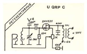
Use the two- tank circuit at input clips of the receivers. It gives you cleaning from unwanted stations and provides your thin Air.
