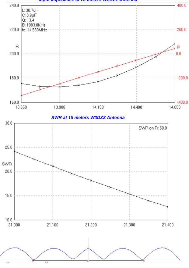
Input Impedance at 20 meters W3DZZ Antenna
