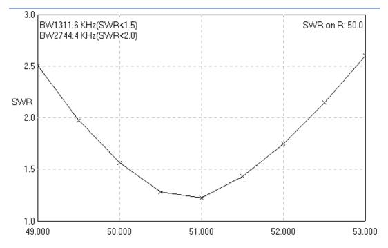
Figure 5 SWR at 50- Ohm coaxial for 'narrow' antenna
