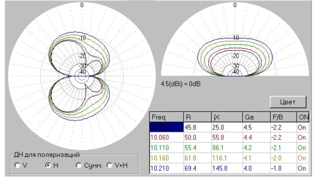
**Comments:** Antenna has strong vertical radiation. Not bad pattern in the vertical plane. Antenna has strong radiation at high corners that allows to do local QSOs. Antenna has almost circular pattern in horizontal plane. Antenna provides DX and local QSOs. Antenna has Z= 55+ j86-Ohms at 1010-kHz. Any ATU does good matching for such load.
