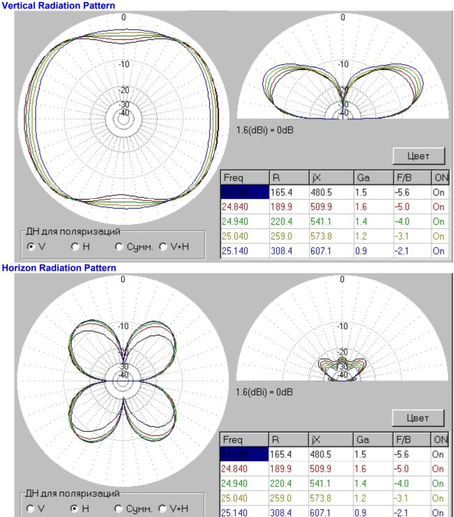
**Comments:** Antenna has strong vertical radiation. A good pattern in the vertical plane. Antenna has almost circular pattern in horizontal plane. Antenna provides DX QSOs. Antenna has Z= 259- j573-Ohms at 25040-kHz. Not all ATUs do good matching for such load.
