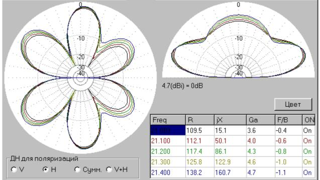
**Comments:** Antenna has both, a strong vertical and strong horizon radiation. For the horizon radiation antenna has a good pattern in the vertical plane with low lobes, and six-lobes pattern in the horizon plane. Pattern for the horizon radiation is not so good as to vertical polarization. Antenna can provide DX QSOs at vertical radiation. Antenna has impedance 117+j86-Ohms at 21200-kHz. Any ATU makes good matching for such load.
