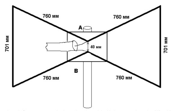
The antenna is made from a copper or aluminum wire in diameter of 4 mm. A copper or brass tube also will do well. The wires fastened by collars to a dielectric plate in 4 mm thickness. I use a plate from PC stuff. The plate fastened by collars to the antenna metal mast. A coaxial cable is connected to points "A" and "B" (the central core to "A", the braid to "B").
