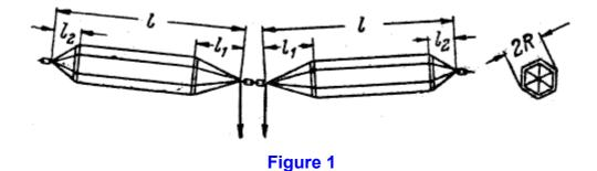
Calculations of input impedance and DD (*for horizon radiation*) of the dipole Nadenenko located at 10 meters above real ground with above mention dimensions (L= 8 meters, L1= 3 meters, L2= 1 meter, 2R= 1 meter, diameter of wires is 2 millimeters) are shown below. You can see, it is possible to use a 50-Ohm coaxial cable with a 1:4 transformer if restricted bands (30, 20, 10 and 6 meters) are used.
