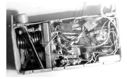
**QRP CW Transceiver. View on to Parts**
