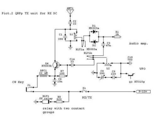
The following version of the transceiver based on receiver (fig. 3) consist in addition keyed freq's doubler and stage of an amplifier. It gives me a good 0.75 watt output at 80 and 40 m bands and 0.3 watt at 20m. I only needed to add the RIT and sidetone.
