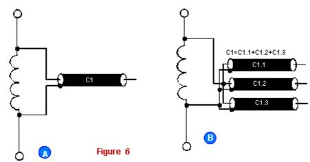
Figure 6 A coaxial cable capacitor
