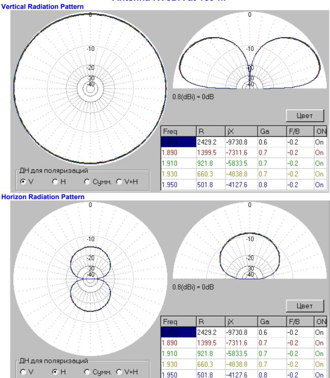
**Comments:** Antenna radiates mainly radio waves with vertical polarization. A very good pattern with low lobes in the vertical plane. Circular pattern in horizontal plane. It is fine for DX- QSO. But antenna has Z= 921-j5833-Ohms at 1910-kHz. Not all ATUs do good matching for such load.
