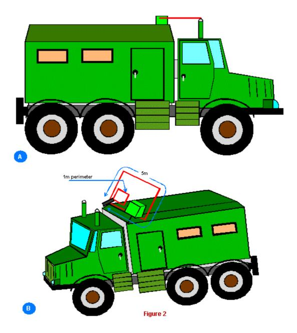
Magnet antenna above the roof of the car cabin
