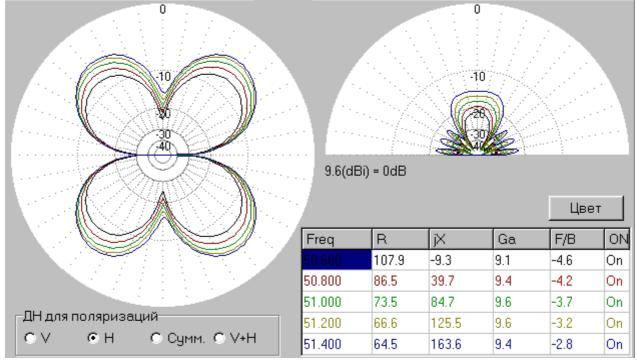
**Comments:** Antenna has strong vertical radiation. A not bad pattern in the vertical plane. Antenna has an "eight- shape" pattern in horizontal plane, so, it demands to choose a proper direction before an installation of the antenna.. Antenna can provide DX QSOs. Antenna has Z= 86+ j40-Ohms at 50800-kHz. The resonance is at the 6- meters band. Any ATU does good matching for such load.
