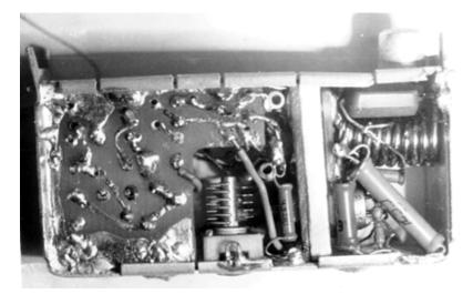
**QRP CW Transceiver. View on the PC Board**
