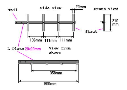
antenna. Boom is made of iron L-plate 25x25-mm. All the four ovals are fastened to the boom by struts made of insulation stuff such as tree, hetinax, etc. Antenna is fastened by the tail, that is behind the struts.
