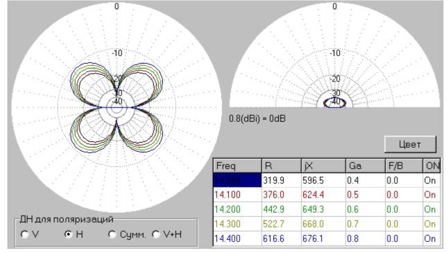
**Comments:** Antenna has strong vertical radiation. A very good pattern in the vertical plane. Antenna has almost circular pattern in horizontal plane. Antenna provides DX QSOs. Antenna has Z= 442+ j649-Ohms at 14200-kHz. Not all ATUs do good matching for such load.
