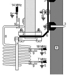
31mm tube (1). The fourth block (bottom) should be drilled with a 5 mm hole to allow water to run out. The bracket is bolted to the balcony handrail, using 35 mm exhaust (muffler) clamps (3).
