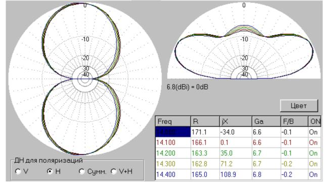
**Comments:** Antenna has strong horizon radiation. A good pattern in the vertical plane. Antenna has a strong radiation at low corners that allows to do DX QSOs. Antenna has almost "eight- figure" pattern in horizontal plane, so, it demands to choose a proper direction before an installation of the antenna. Antenna provides DX QSOs. Antenna has the resonance at 14100-kHz at 166 Ohms. Any ATU does good matching for the antenna.
