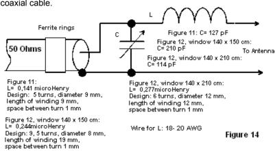
Figure 14 Matching device for antenna with capacitive loads
