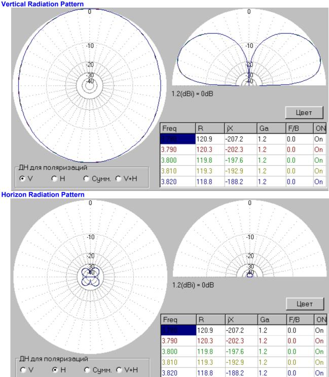
**Comments:** Antenna radiates radio waves with vertical polarization. A very good pattern with low lobes in the vertical plane. Circular pattern in horizontal plane. It is fine for DX- QSO. Antenna has Z= 119-j197-Ohms at 3800-kHz. Almost any ATU does good matching for such load.
