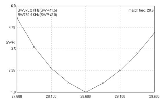
Figure 15 SWR at 50- Ohm coaxial connected through a matching device (see Figure 14) to antenna shown at Figure 11
