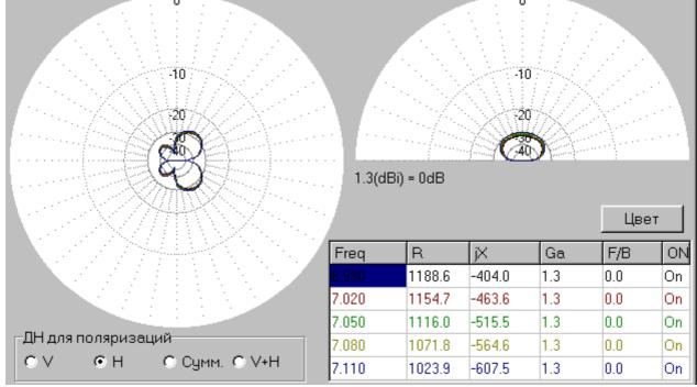
**Comments:** Antenna radiates radio waves with vertical polarization. A very good pattern with low lobes in the vertical plane. Almost a circular pattern in horizontal plane. It is fine for DX- QSO. Antenna has Z=1116- j515-Ohms at 7050-kHz. Not all ATUs do good matching for such load.
