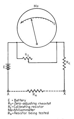
FIG. 4-13.—Basic ohmmeter circuit.
