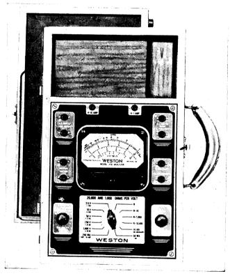
FIG. 4-1.—The Weston Model 772 multimeter.
