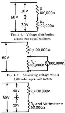
FIG. 4-8.—Voltage distribution resulting from loading the circuit with a 1,000-ohmsper-volt meter.
