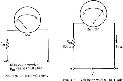
Fig. 4-3.—Voltmeter with 0- to 1-volt range at full-scale deflection.
