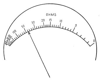
FIG. 4-14.—Typical ohmmeter scale.
