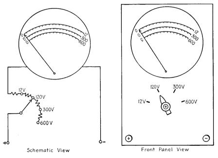
FIG. 4-5.-Multirange voltmeter showing range switch.
