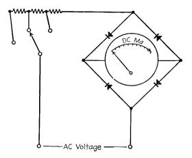
FIG. 4-12.—Typical multirange AC voltmeter.
