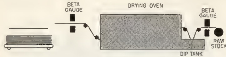
Fig. 2.2 Horizontal treater. (General Electric Company.)
