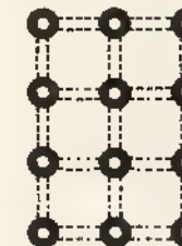
Fig. 19.37 Test coupon used for plated-through-hole structure testing (IPC).
