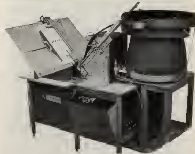
Fig. 11.20 The machine shown here receives loose DIPs out of a plastic stick, performs a spreading, straightening operation on the leads, and assembles the DIP into a unit carrier fed from the vibratory bowl. The loaded carrier is then fed into magazines holding 25 each.
