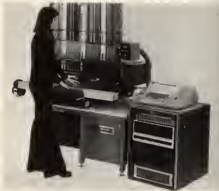
Fig. 11.30 Sequencer-Inserter combination machine. Input capacity is 48 magazines of DIP sticks.
