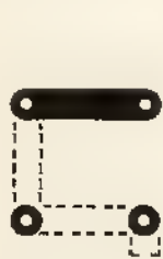
Fig. 19.39 Continuity, thermal stress, current-carrying capacity, and moisture resistance test pattern (IPC).
