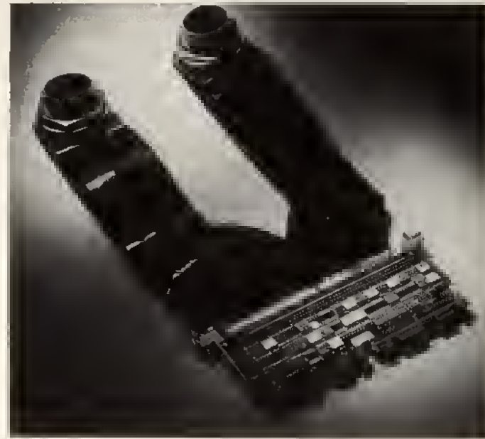
Fig. 24.7 Multilayer flexible printed circuit assembly (IBM).
