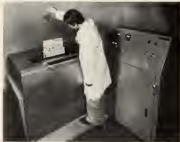
Fig. 14.6 Hot-air solder-leveling machine. (Courtesy Electrovert, Inc.)
