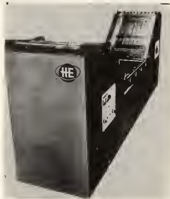
Fig. 16.9 In-line conveyorized vapor cleaner. In-line cleaning lends itself well to high-volume production.
