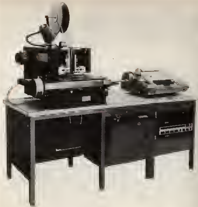
Fig. 11.29 VCD insertion system with computer control. A typical assembled board is shown in Fig. 11.14.
