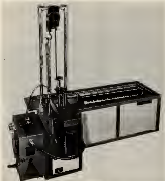
Fig. 15.7 Wave-Solitar pot with nozzle and automatic solder level control (Electrocraft, Inc.).
