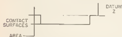
Fig. 4.1 Definition of contact surfaces. (1) Contact surfaces are defined as those shown in low datum Z and in the applicable drawing. (2) The amount of plated copper at datum Z should be kept to a minimum.
