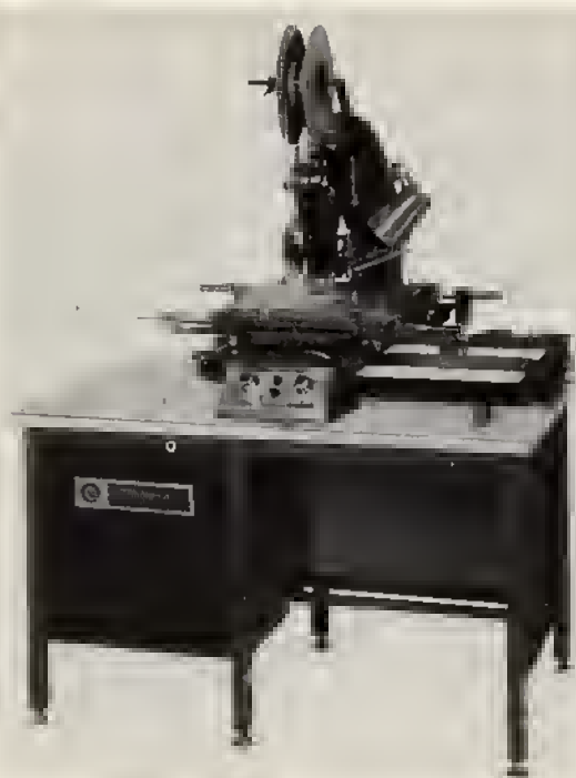
Fig. 11.22 Single-station manual pantograph board-locating insertion machine. Best economy is obtained when several units of a specific component are inserted into a given board in one setup.
