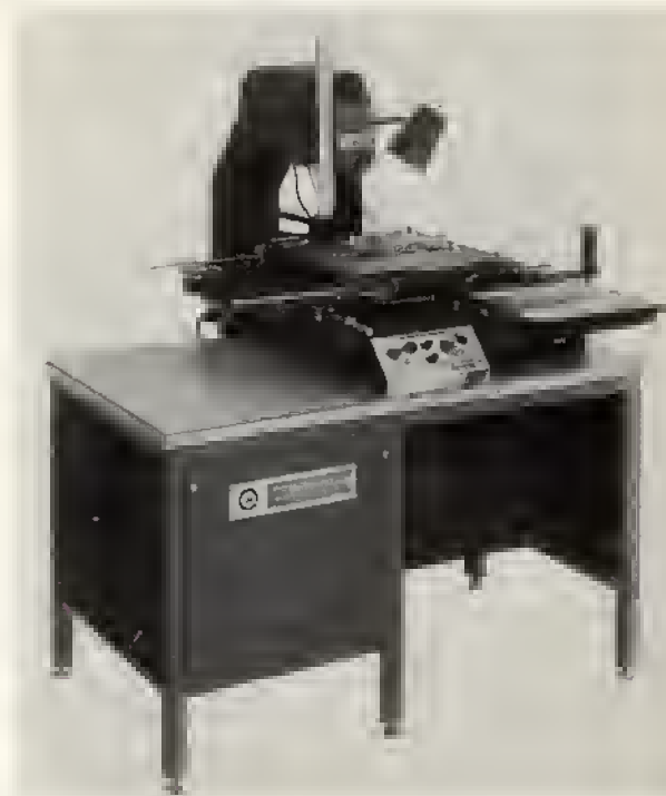
Fig. 11.23 Pantograph system for insertion of a single type of DIP from a magazine input.
