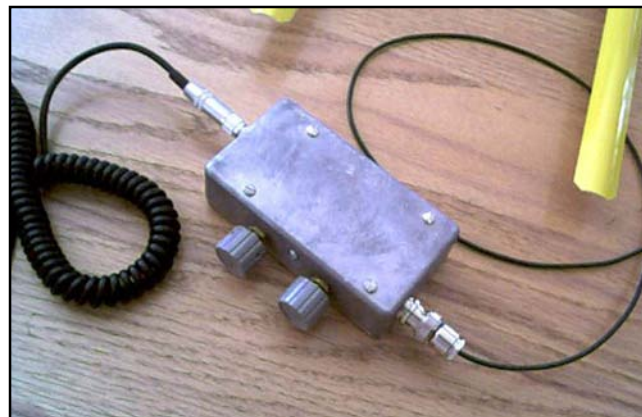
Fig 3—The 318 MHz receiver. The controls are for regeneration and volume.
