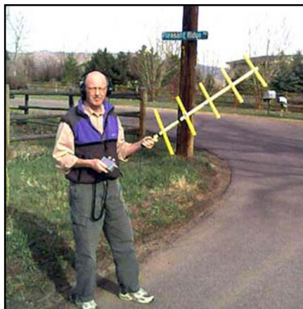
Fig 1—The author searching for power-line noise.
