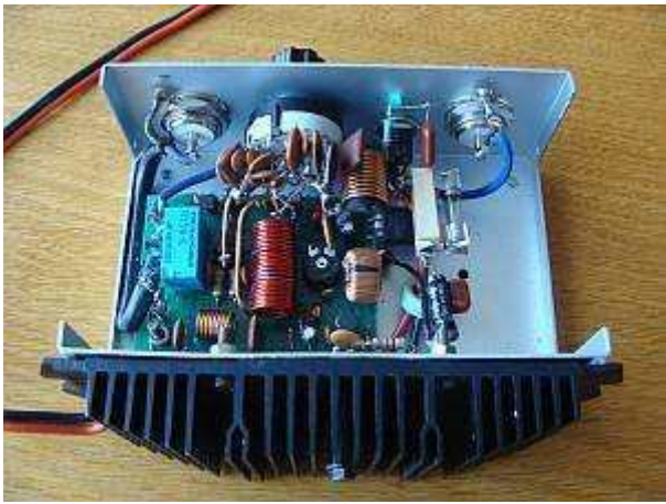
The 5-band HF power amplifier "insides"
